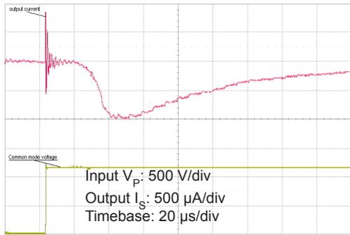
Figure 11: Typical common mode perturbation (1200 V step with 6 kV/µs  $R_M = 100 \Omega$ )
